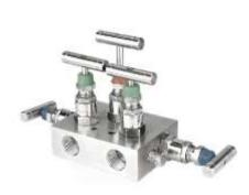
Manifolds have been designed for use with differential pressure transmitters to measure fluid flow using primary elements and fluid levels on the principle of differential pressure. 5-way valve sets (for water or steam) or 3-way valve sets (for air and gases) allow for easy connections to pressure outlets, simplifying continuous cleaning of impulse pipelines. Manifolds are available in stainless steel, brass, steel, Monel, bronze, Hastelloy C, Incoloy, and Inconel 600.
