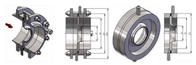
Nozzle with pressure tappings - welded
