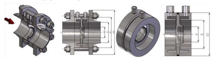
Nozzle with chamber tappings - welded
